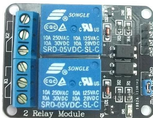
Figure 19.1 Opto-Isolated, 2 Channel Relay Module.
