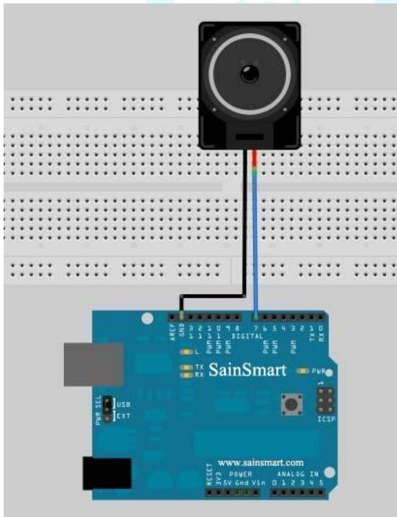
**Figure 7.2** Passive buzzer experiment connection.
