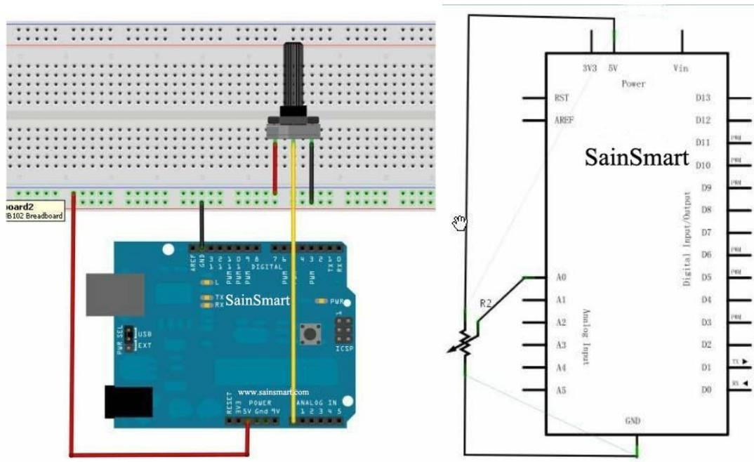
Figure 10.1 Potentiometer sketch circuit.
