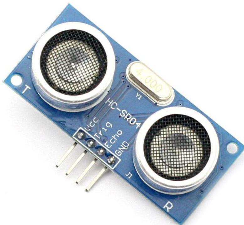
**Figure 20.1** Ultrasonic ranging module HC-SR04
