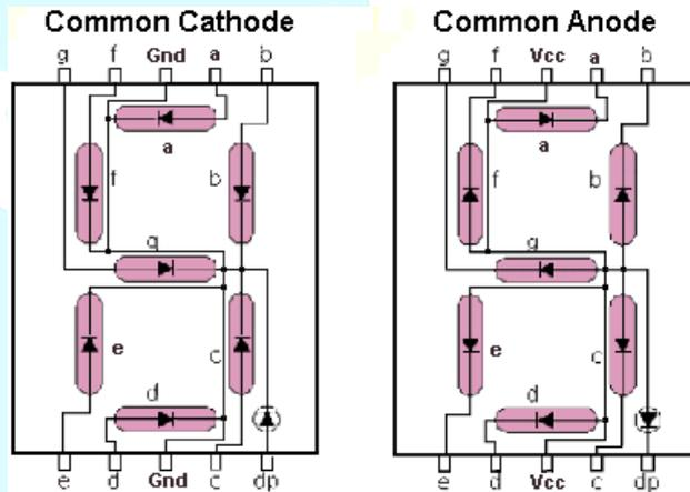
Figure 13.2 Common Cathode and Anode pinouts. (Source: www.thelearningpit.com)
