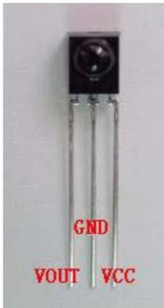
**Figure 17.1** IR receiver module.
