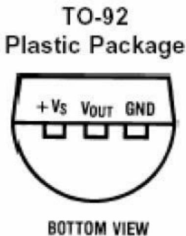
Figure 12.2 LM35 Pinout.
