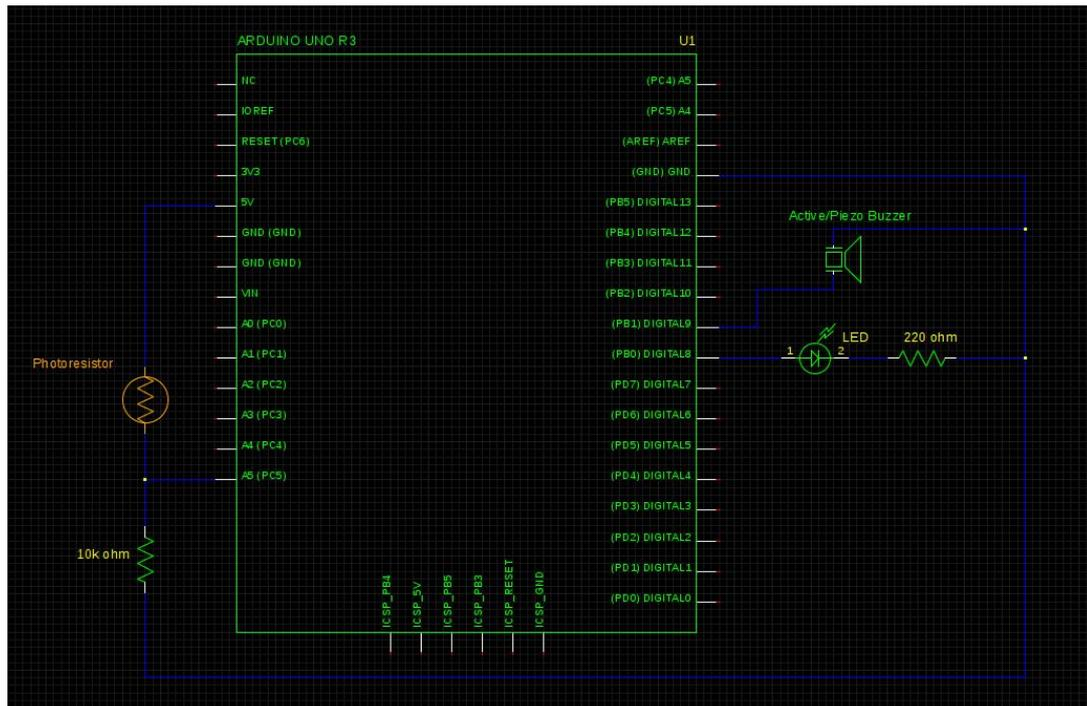
**Figure 11.2** Photoresistor sketch circuit.
