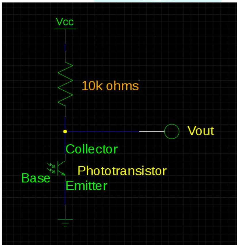
**Figure 8.3** Phototransistor common-emitter amplifier circuit.
