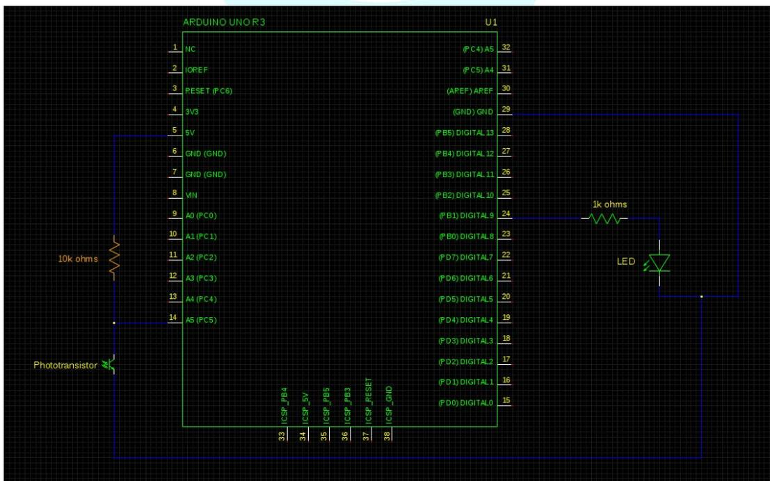
Figure 8.4 Schematic of the fade2 sketch circuit.
