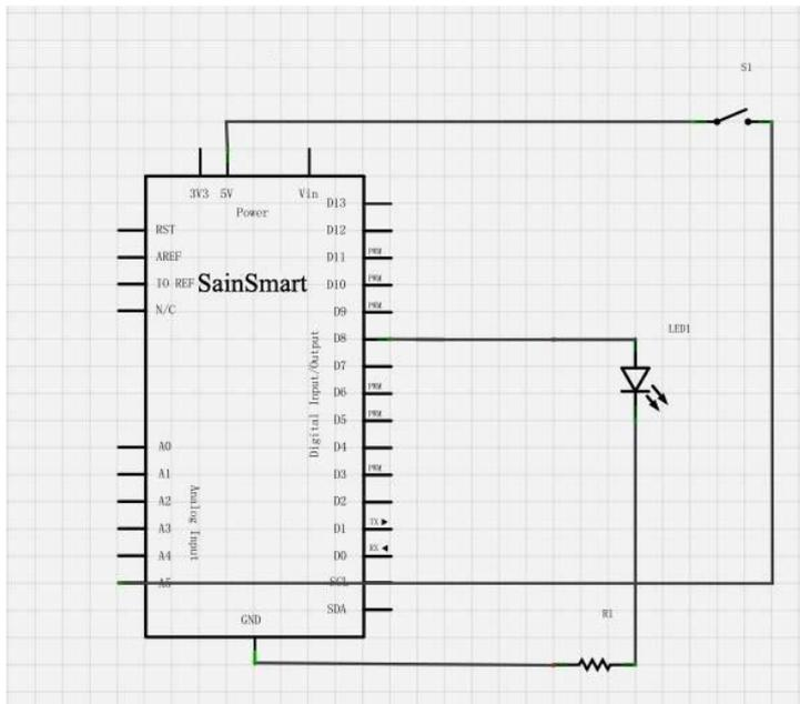
**Figure 9.2** Schematic for tilt sensor-LED sketch circuit.
