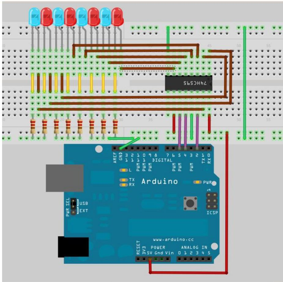
**Figure 15.4** Circuit for the LED light pattern sketch.
