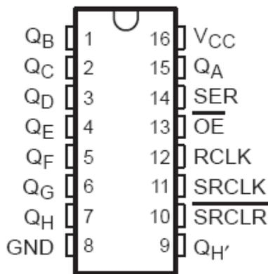
**Figure 15.1** Pin assignments for the 74HC595.
