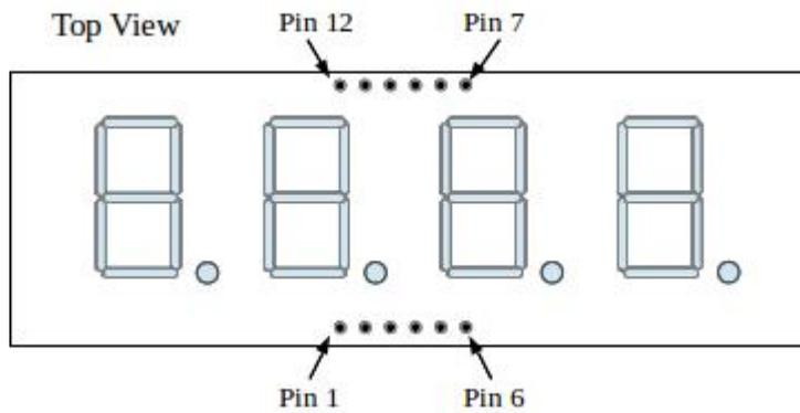
Figure 14.3 Pin numbers for the 4-digit, 7-segment display.
