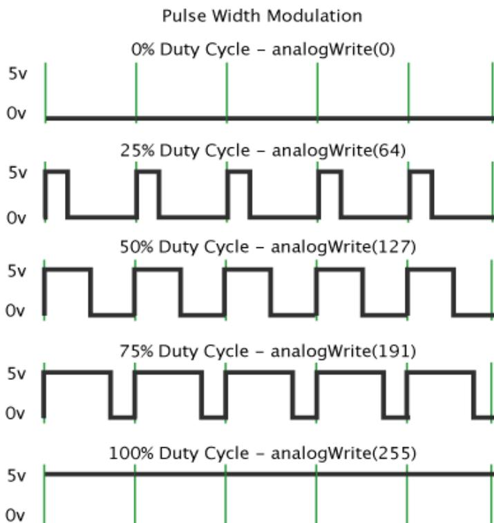
Figure 5.1 Pulse width modulation waveforms.
