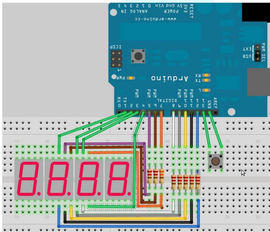
Figure 14.4 Stopwatch circuit for the 5643A type package.
