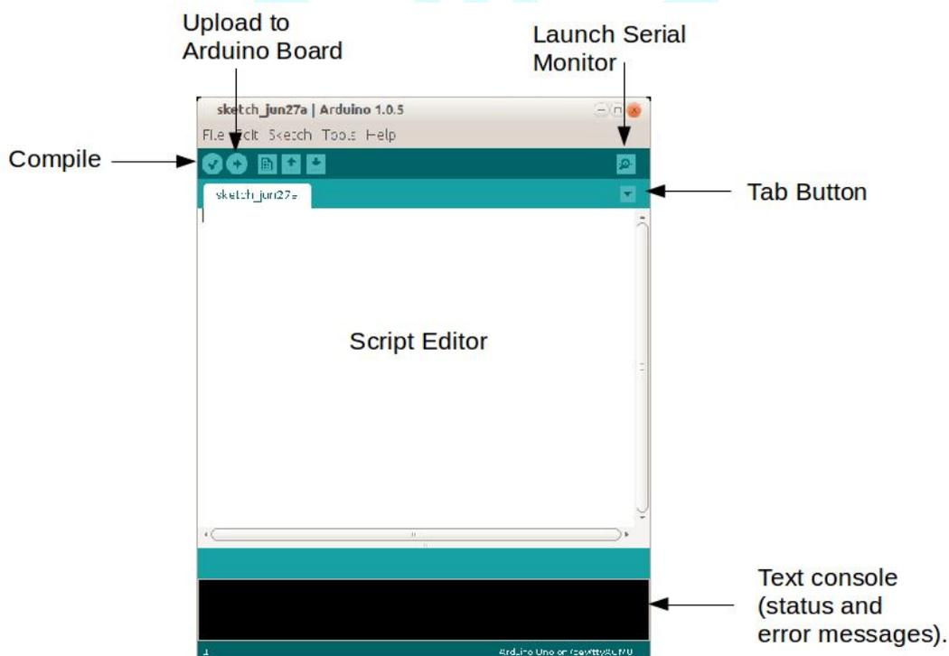
**Figure 1.1** The Arduino IDE.
