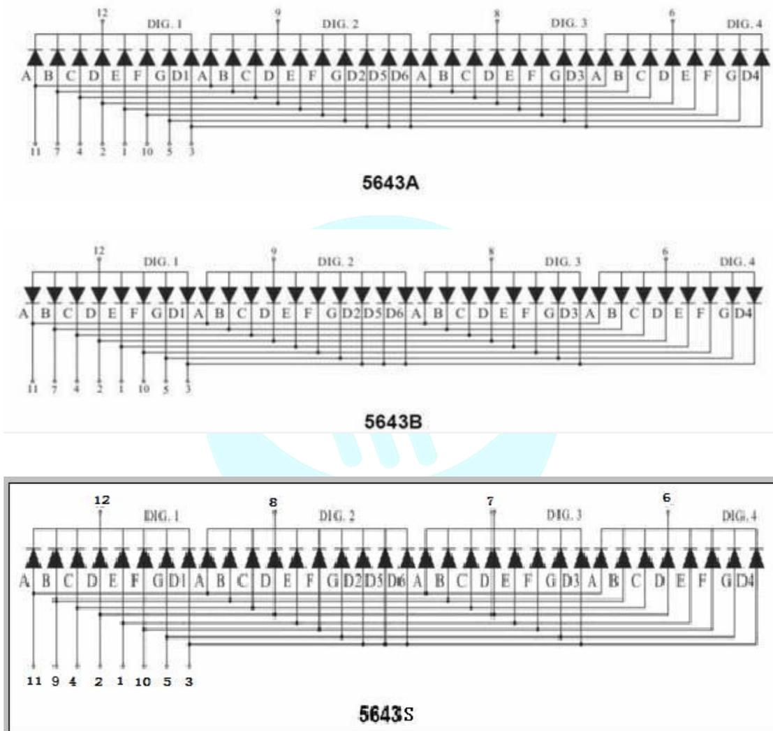
**Figure 14.2** Pinouts for various types of multi-digit, 7-segment displays.
