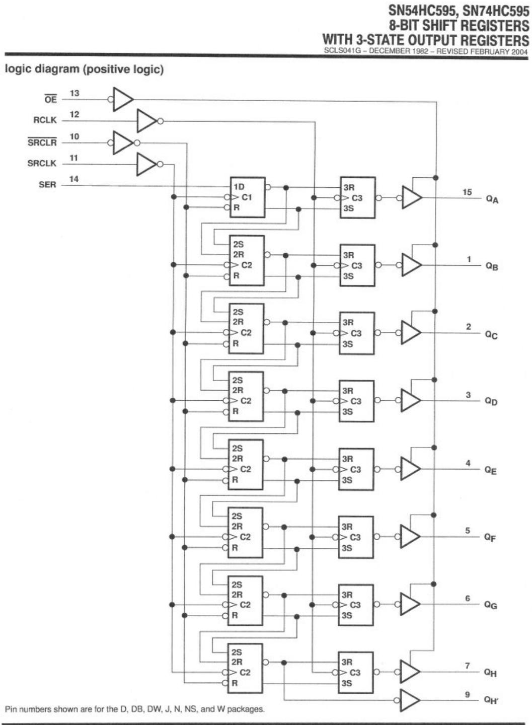
**Figure 15.2** Logic diagram of the 74HC595.
