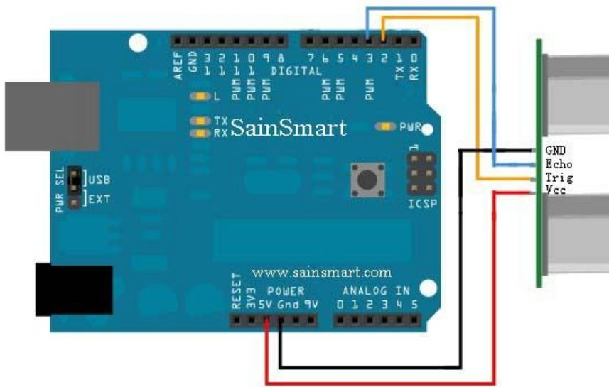
Figure 20.2 Distance sketch connections.
