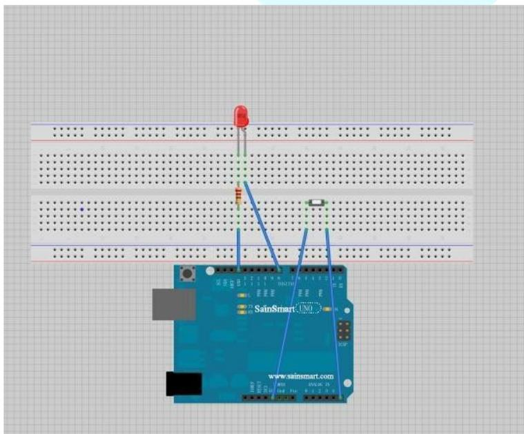
**Figure 9.3** Illustration of tilt sensor-LED sketch circuit.
