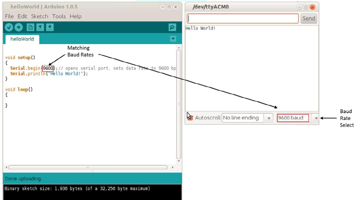
**Figure 3.2** The helloWorld sketch window (left) and the Serial Monitor window (right), shown with matching baud rates of 9600.
