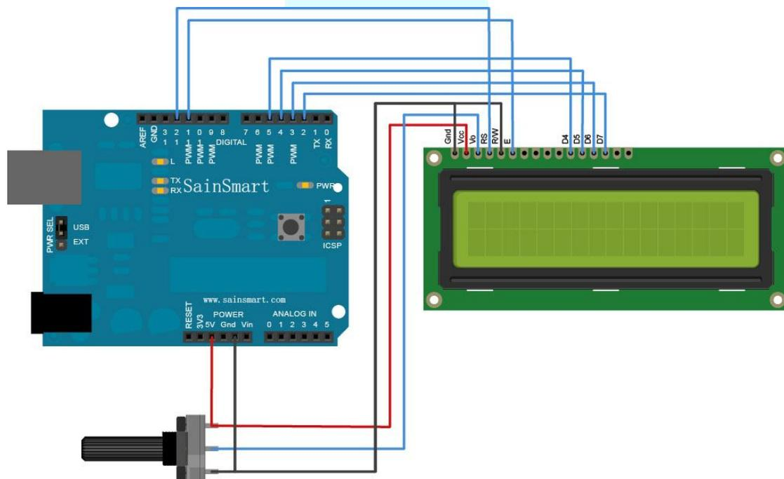
**Figure 18.2** Drawing of the 1602 LCD and Uno connection for the LiquidCrystal sketches.
