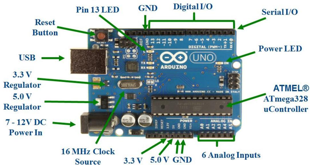
Figure 1.2 Arduino Uno, R3 board.
