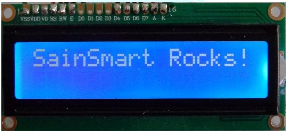
**Figure 18.1** The 1602 LCD module
