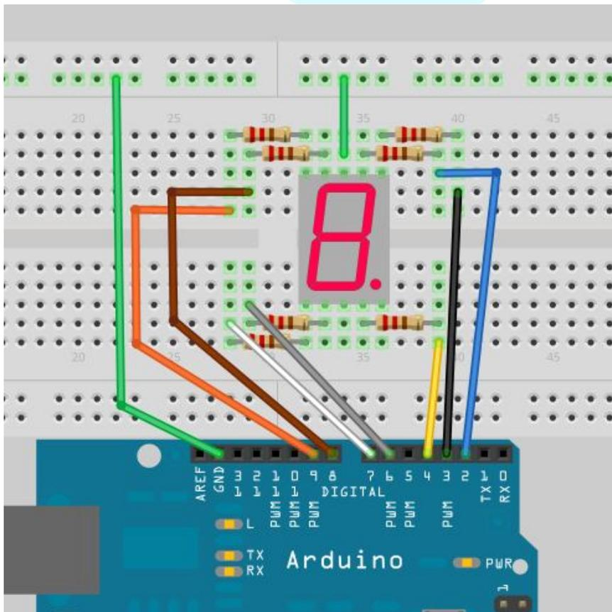
**Figure 13.2** Seven segment display connected to the Uno.
