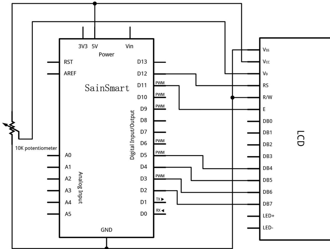
Figure 18.3 Schematic of 1602 LCD and Uno for the LiquidCrystal sketches.
