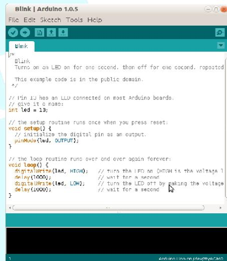
Figure 2.2 The Blink sketch in a new window.
