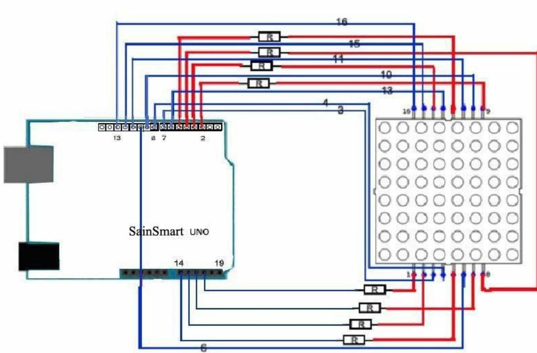
Figure 16.2 Wiring for the letter display sketch.
