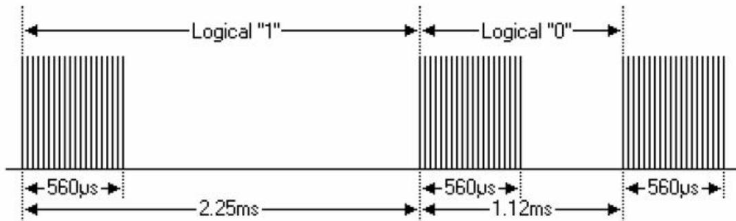
**Figure 17.2** A logic “1” and logic “0” for the NEC protocol.
