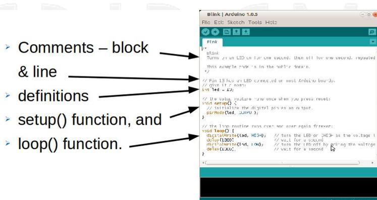
Figure 2.3 The four basic parts of an Arduino sketch.
