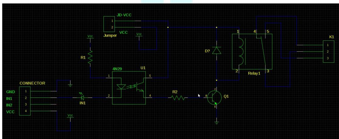
Figure 19.2 Schematic of 1-channel of the 2-channel relay board.
