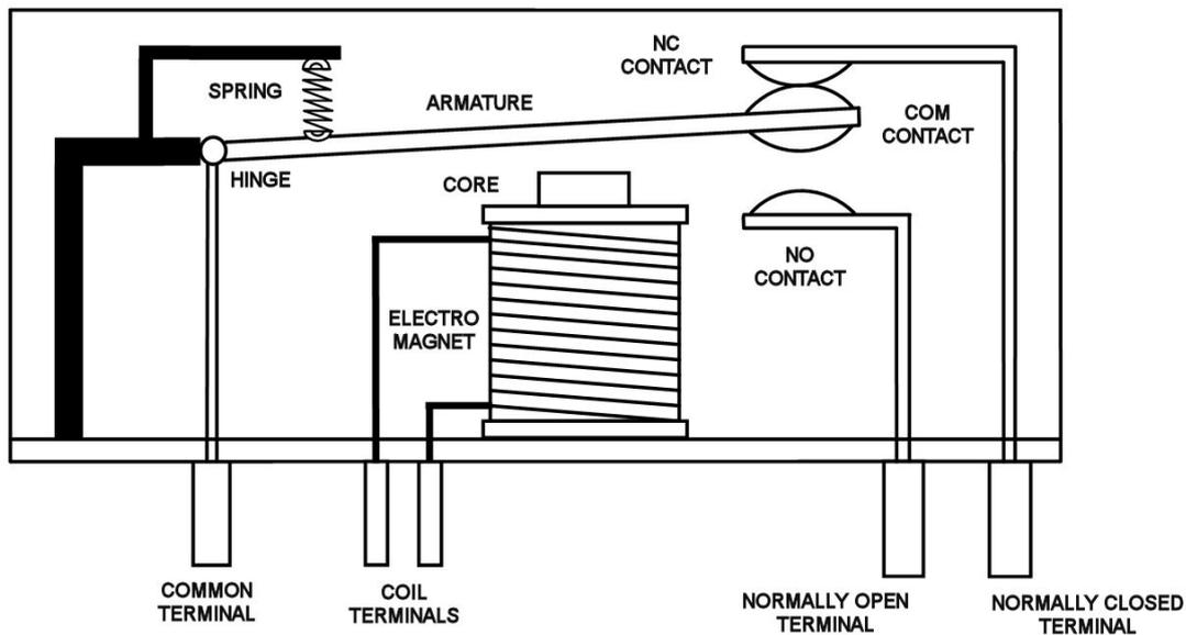
**Figure 19.3** The internals of a two contact relay.
