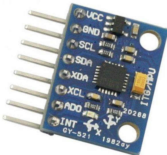
**Figure 23.1** Blown up view of the MPU-6050 sensor.
