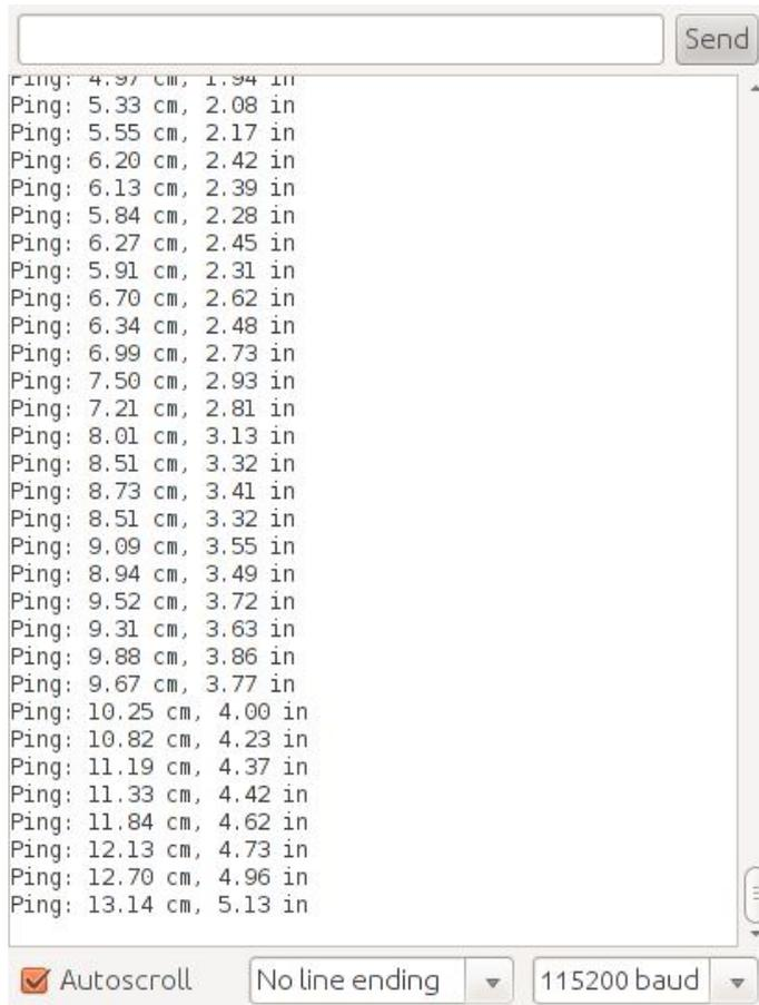
**Figure 20.4** Distance sketch data in the Serial Monitor window.
