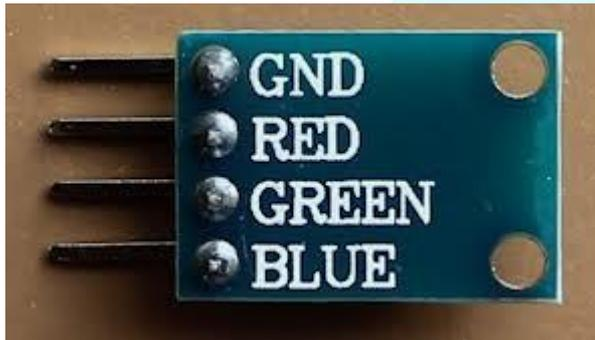
**Figure 6.1** Tri-color LED module – backside.
