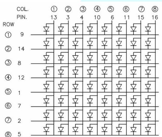
Figure 16.1 8x8 Dot LED matrix display schematic.
