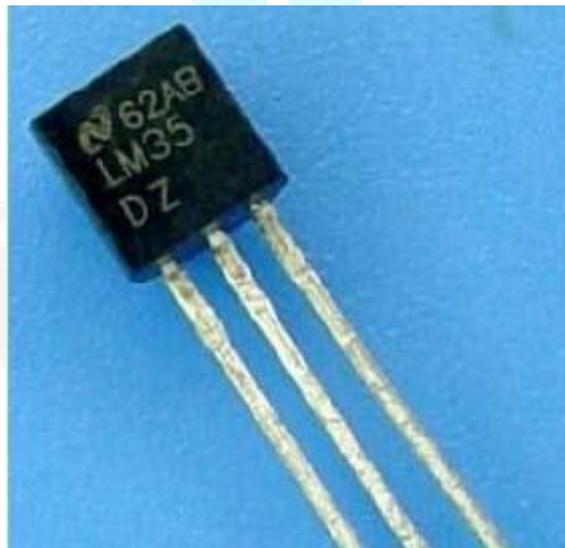
**Figure 12.1** LM35 Precision Centigrade Temperature Sensor.
